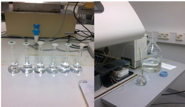
Figure 2. ICP-OES analysis in the laboratory showing prepared test and standard (calibration) solutions.
